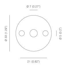
Mounting screws not included. 5mm countersunk screw recommended.
