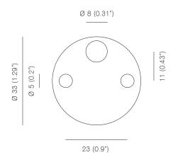
Mounting screws not included. 5mm countersunk screw recommended.
