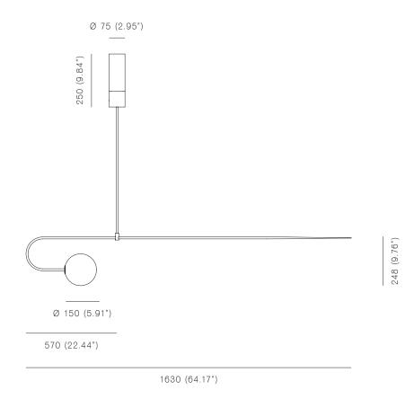
$66.35\ 50W\ /\ 12V$  frosted halogen for ø150mm sphere  $760\ \text{Im}\ /\ 2700\text{K}$
