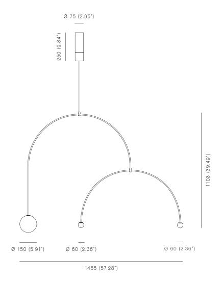
$66.35\ 50W\ /\ 12V$  frosted halogen for ø150mm sphere  $760\ \text{Im}\ /\ 2700\text{K}$
