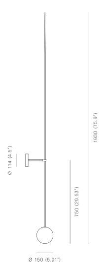
Bulb specifications 240V G9 40W frosted halogen bulb 460 lm / 2800K
