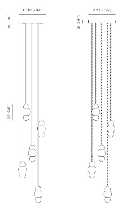
Bulb specifications 240V E14 G9 33W Raxon halogen retrofit / ø45mm white globe 458 lm / 2700K
