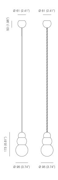
Bulb specifications 240V E27 G9 33W Raxon halogen retrofit / ø95mm white globe 458 lm / 2700K
